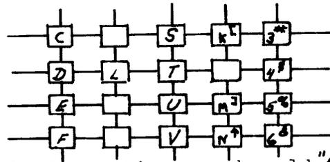
*Note: Simply shift common connection of keys "K", "M", and "N" to common of keys "X", "Y", and "Z".*
