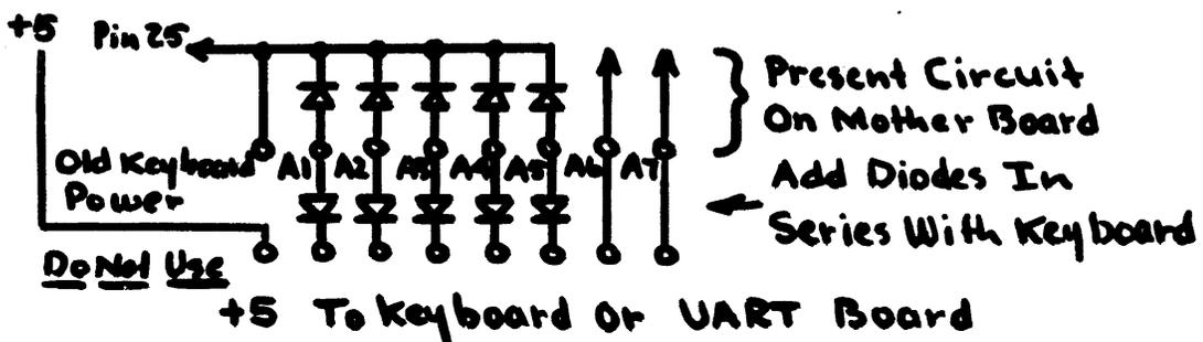
NOTE THAT THE KEYBOARD POWER SUPPLY IS NOW PERMANENTLY CONNECTED TO THE +5 SUPPLY. IT DOES NOT HURT THE KEYBOARD OR UART BOARD NOW TO HAVE A1 THRU A5 GROUNDED.
