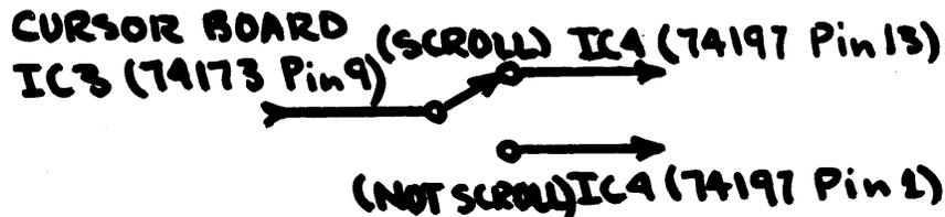
IF ONLY SCROLLING IS TO BE USED, PIN 9 OF IC3 CAN BE PERMANENTLY CONNECTED TO PIN 13 OF IC4. FINALLY, MAKE THE CHANGE SHOWN BELOW TO THE INPUT ON THE MOTHER BOARD. (THIS CHANGE SHOULD BE MADE TO THE INPUT EVEN WITHOUT THE SCROLLING BEING USED IF THE UART BOARD DESCRIBED IN R-E, FEB 1975 IS USED AS HE CLEARS THE INPUTS BY SHORTING THE OUTPUTS OF THE 74157 MULTIPLEXERS TO GROUND WHICH IS A VERY BAD PROCEDURE.)
